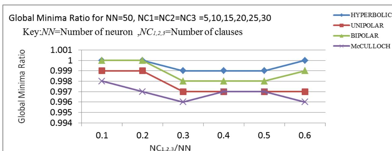
**Figure 6:** Global minima ratio for hyperbolic tangent activation function, unipolar activation function, bipolar activation function and McCulloch-Pitts function for  $NC_{1,2,3}=5,10,15,20,25,30$  and given  $NN = 50$
