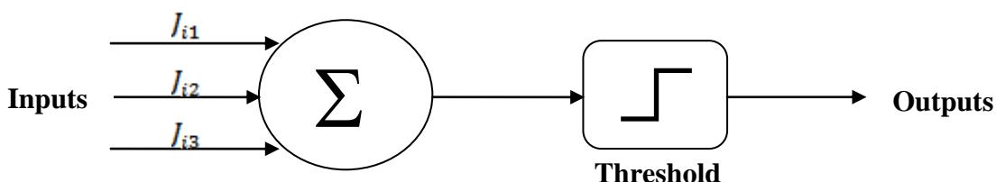
**Figure 4:** Schematic diagram of a McCulloch-Pitts neuron model [9].
