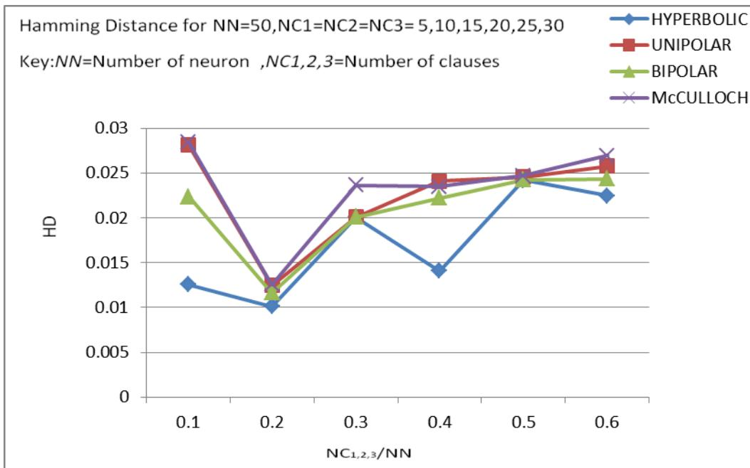
**Figure 7:** Hamming Distance for hyperbolic tangent activation function, unipolar activation function, bipolar activation function and McCulloch-Pitts function for  $NC1,2,3=5,10,15,20,25,30$  and given  $NN=50$  for  $NC$  given  $NN = 40$
