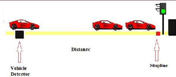
**Fig-2: SCOOT Vehicle Detectors
