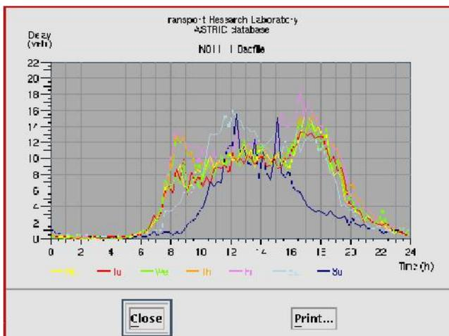
Fig-6: Historic database of key link and detector based values Generated by SCOOT
