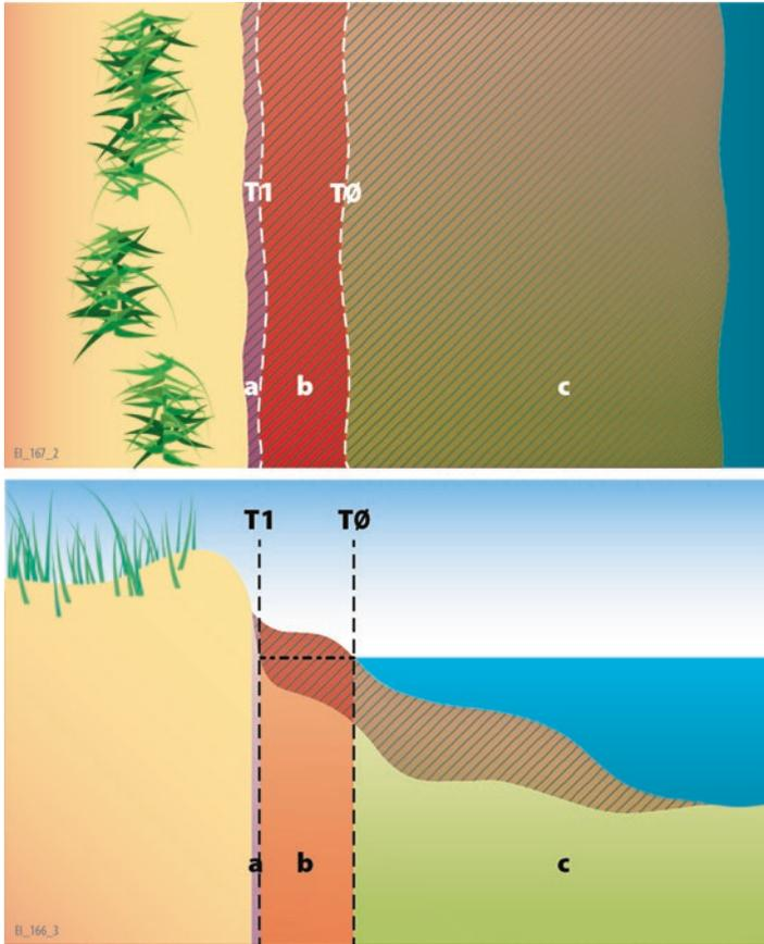
**Fig. 12.2** Schematic of an eroded beach profile. Shoreline change is the horizontal difference between  $T_0$  and  $T_1$ . Volume change is the vertical difference within the hashed areas of  $a$ ,  $b$  and  $c$
