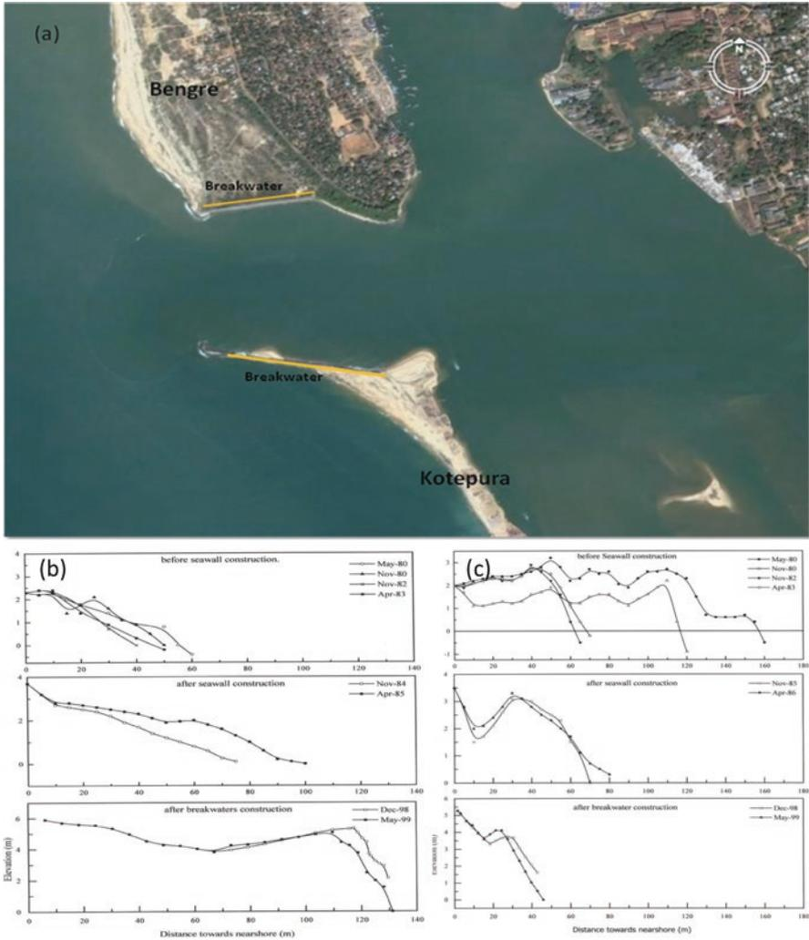
**Fig. 21.2** Showing deposition of sediment and widening of Bengre Beach on the up-drift side and erosion of Kotepura Beach on the down-drift side of breakwaters (a), Seasonal beach profiles of Bengre (b), and Kotepura (c). (Source: Jayappa and Vijaya Kumar 2003)
