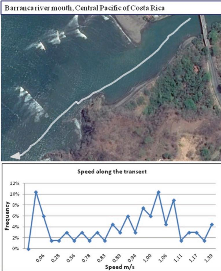
**Fig. 22.15** Trajectory of a river mouth current traced by a current meter at Barranca river mouth (Costa Rica). The length from the bridge to the arrow is approximately 580 m
