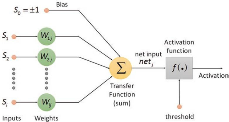
Fig. 10.4 Artificial Neural Network structure
