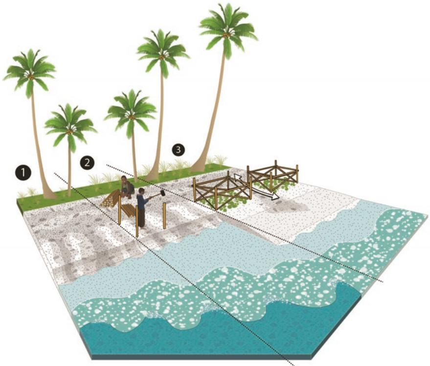
**Fig. 34.6** Steps in construction of access control. (1) Assess causes of beach erosion and consult with the community. (2) Use poles and rope to build a fence on the upper beach. (3) maintain the access control and inform the local community regarding its purpose
