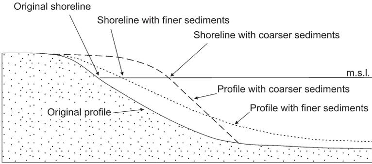
**Fig. 15.11** At parity of volume, coarser sediments produce a wider subaerial beach than finer ones. An offshore profile shift is given by sediments of the native ones size
