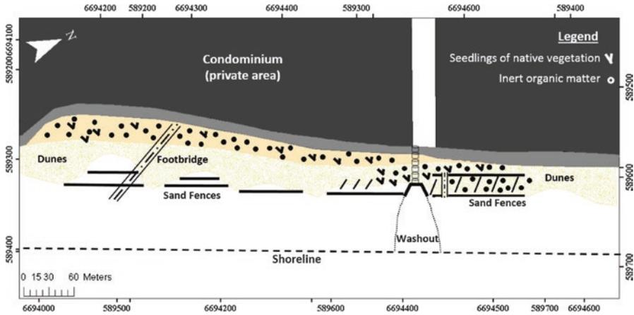
Fig. 3.2 Layout of the restoration measures in the foredune
