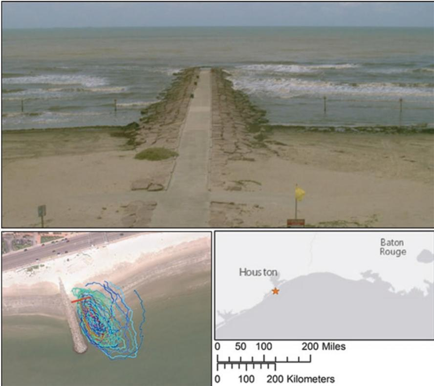
**Fig. 24.10** Photograph of structurally-controlled rip current on the left-side of the groin, creating a strong circulation cell (*bottom right image*). The groins are placed at regular intervals along the Galveston Seawall to protect the seawall from erosion. Primary access points are located at the center of each groin leading to the employment of warning signs and lifeguard stands at each access point to reduce the risk to the public
