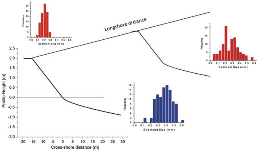
**Fig. 13.1** Idealized 3D beach. Emerged part based on real data from Mexican beaches. Immersed part based on Dean’s equilibrium profile form. Three different sediment distribution used in cross-shore and longshore dimensions. Vertical scale exaggerated
