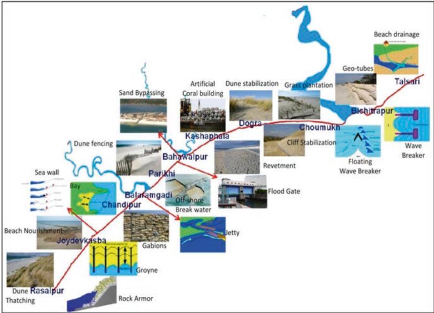
**Fig. 38.6** Proposed installation places of different hard and soft coastal engineering structures
