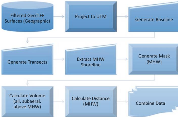
**Fig. 12.1** Data processing model for extracting metrics from LiDAR data
