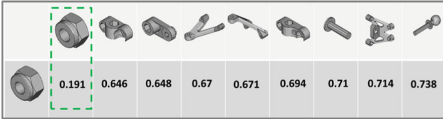
Fig. 62.4 Complex Chassis assembly: dissimilarity values of nine part examples W.R.T. p^{(45)} are shown in the figure. only one part with a dissimilarity value of 0.191 is detected as a similar part
