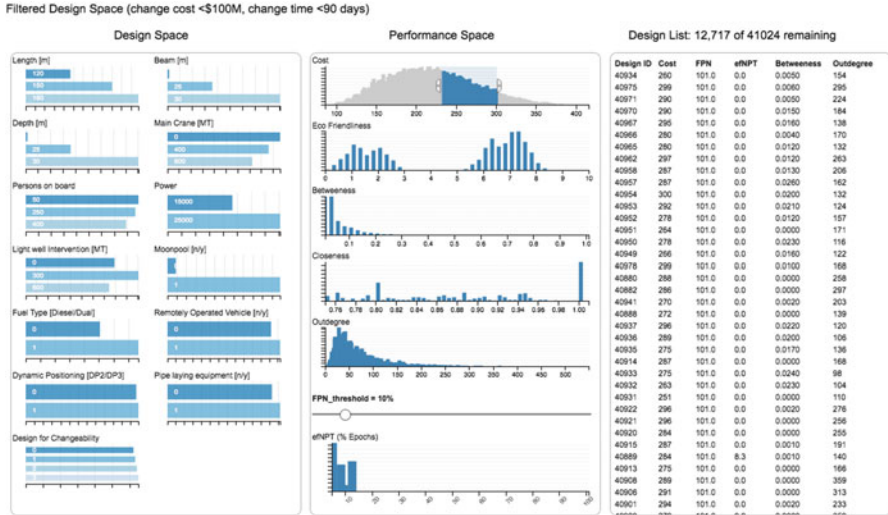
Fig. 19.5 Interactive filtering application implementing OLAP for the offshore case (Filtered for allowable change cost <$100 M and change time <90 days)
